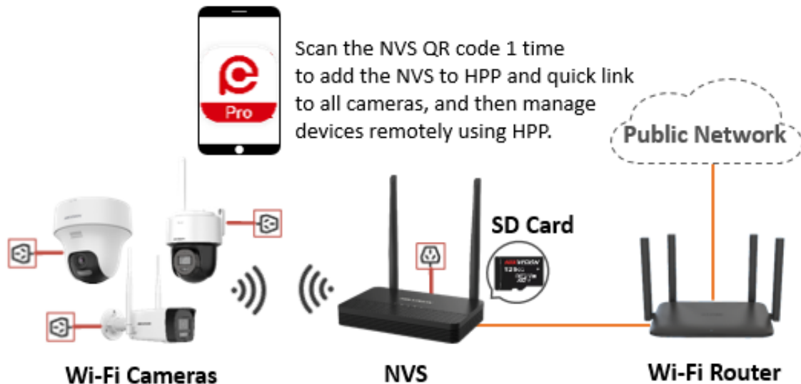
Figure 44-1 Typical Application: Wireless Video Management with Hik-Partner Pro & EasyLink Wi-Fi Kit
